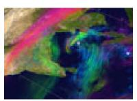
Genesis of the very severe cyclonic storm Nargis (2008) associated with the equatorial Rossby wave: (a) A pair of low-level vortices at 96h simulation (labeled with 'V') indicate formation of the Rossby wave. Cyclone Nargis formed when the northern vortex strengthened. (Bryan Green, NASA/Ames; Bo-wen Shen, NASA/Goddard)
