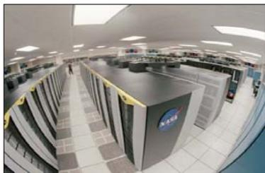
The Columbia supercomputer with (in late 2004): (1) 20 SGI Altix superclusters, each with 512 CPUs; (2) 10,240 Intel Itanium II CPUs; (3) 20 TB total memory with 1 TB of memory per 512 CPUs (Biswas et al., 2007).
