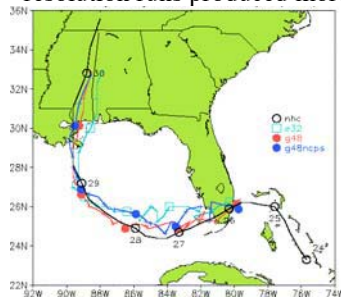
Figure 1: Track forecasts for Hurricane Katrina (2005) from 5-day simulations initialized at 1200 UTC August 25, 2005 with the global mesoscale model at different resolutions: e32 (0.25°), g48 (0.125°), and g48ncps (0.125° without CPS)
